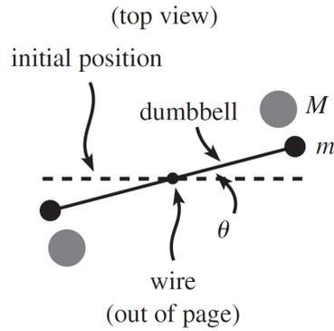
The masses produce attractive forces on the dumbbell masses and cause the dumbbell to twist counterclockwise. The dumbbell will oscillate back and forth before finally settling down at some tiny angle away from the initial position.
