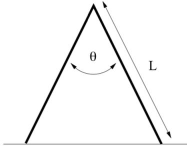
The sign shown below consists of two uniform legs attached by a frictionless hinge. The coefficient of friction between the ground and the legs is  $\mu$ . Which of the following gives the maximum value of  $\theta$  such that the sign will not collapse?
