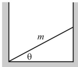
A uniform stick with mass  $m$  is placed in a frictionless well. The angle the stick makes with the horizontal is  $\theta$ , as shown in the diagram. What are the forces the well exerts on the stick at its two ends?
