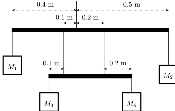
In the mobile below, the two cross beams and the seven supporting strings are massless. The hanging objects are  $M_1 = 400 \text{ g}$ ,  $M_2 = 200 \text{ g}$ , and  $M_4 = 500 \text{ g}$ . What is the value of  $M_3$  for the system to be in static equilibrium?
