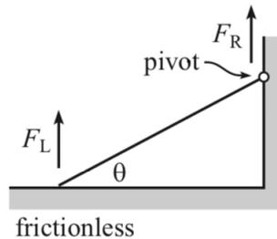
One end of a stick with mass  $m$  and length  $l$  is pivoted on a wall, and the other end rests on a frictionless floor, as shown in the diagram. Let  $F_L$  and  $F_R$  be the vertical forces on the left and right ends of the stick, respectively. Then
