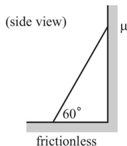
A ladder leans against a wall at a  $60^\circ$  angle, as shown in the diagram. The floor is frictionless, but there is friction with the wall. Assume that the coefficient of friction is large (say,  $\mu = 10$ ). Is it possible for this setup to be static?
